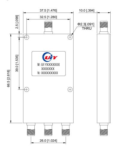
Unit: mm/ inch, General part tolerance is ±2% unless otherwise stated.
