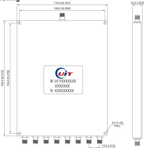
Unit: mm/ inch, General part tolerance is ±2% unless otherwise stated.
