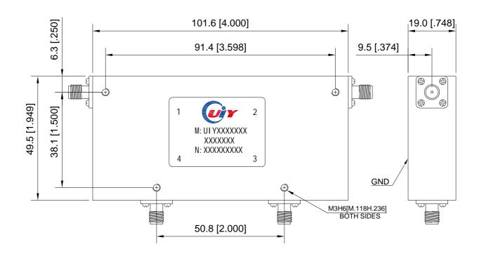
Unit: mm/ inch, General part tolerance is ±2% unless otherwise stated.
