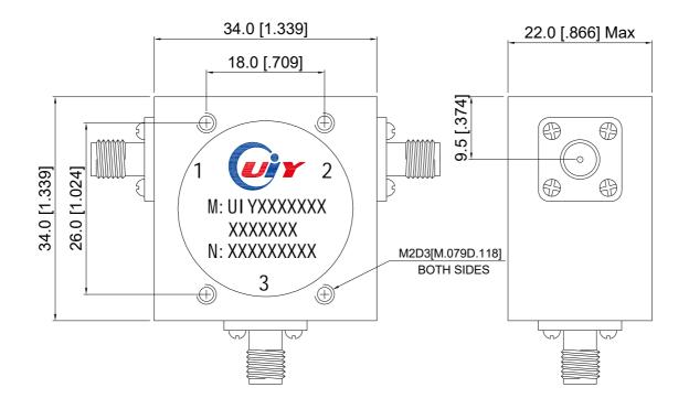
Unit: mm/ inch, General part tolerance is ±2% unless otherwise stated.
