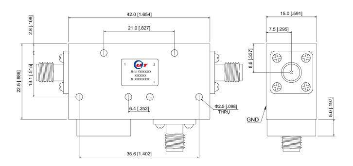
Unit: mm/ inch, General part tolerance is ±2% unless otherwise stated.
