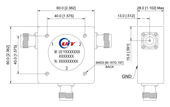
Unit: mm/ inch, General part tolerance is ±0.2mm unless otherwise stated.
