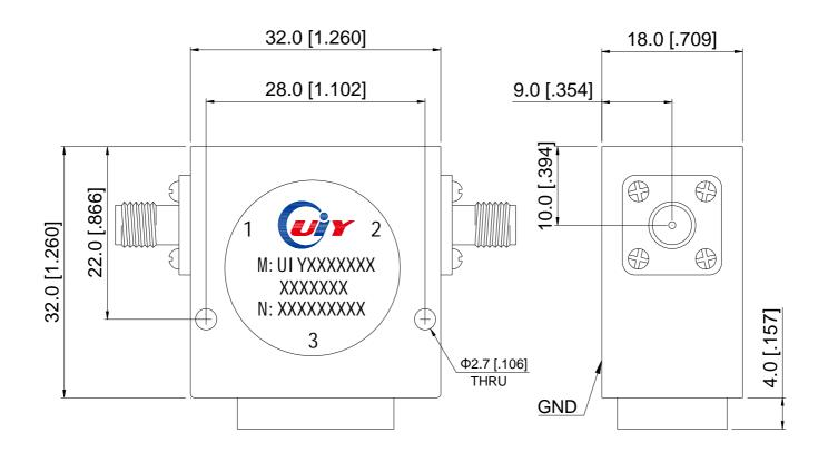
Unit: mm/ inch, General part tolerance is ±0.2mm unless otherwise stated.
