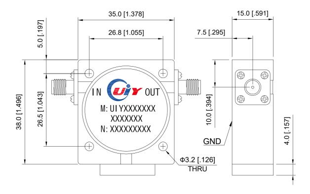
Unit: mm/ inch, General part tolerance is ±2% unless otherwise stated.
