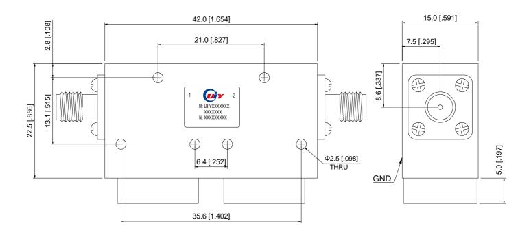
Unit: mm/ inch, General part tolerance is ±0.2mm unless otherwise stated.
