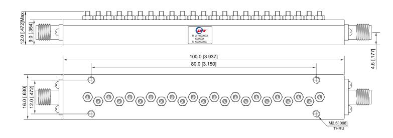
Unit: mm/ inch, General part tolerance is ±2% unless otherwise stated.
