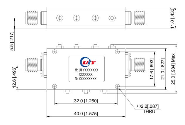
Unit: mm/ inch, General part tolerance is ±2% unless otherwise stated.
