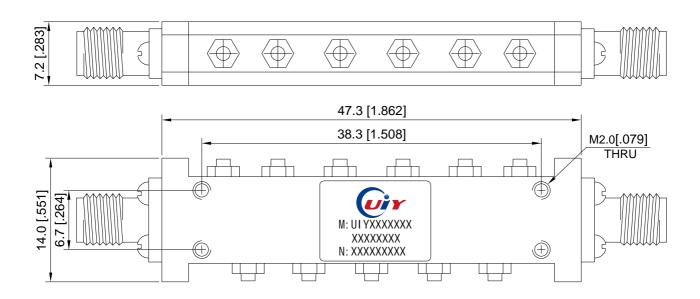
Unit: mm/ inch, General part tolerance is ±2% unless otherwise stated.
