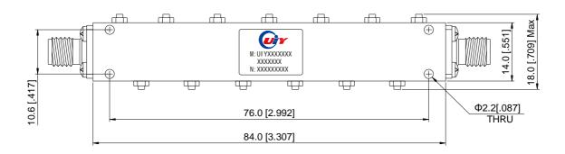
Unit: mm/ inch, General part tolerance is ±2% unless otherwise stated.
