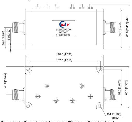
Unit: mm/ inch, General part tolerance is ±2% unless otherwise stated.
