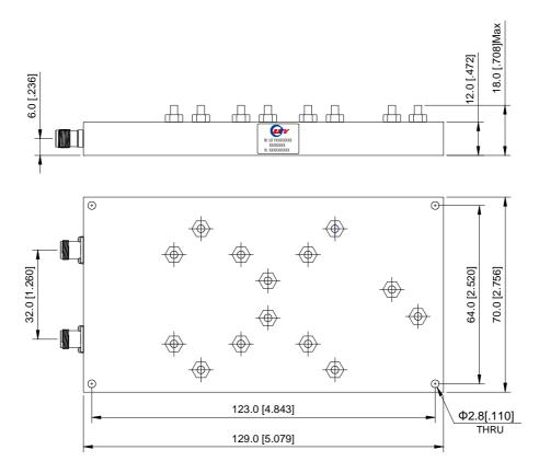
Unit: mm/ inch, General part tolerance is ±0.2mm unless otherwise stated.
