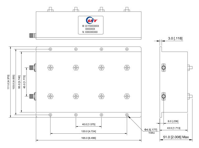
Unit: mm/ inch, General part tolerance is ±2% unless otherwise stated.
