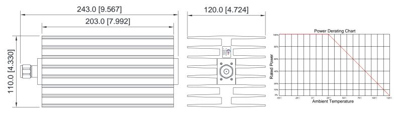
Unit: mm/ inch, General part tolerance is  $\pm 2\%$  unless otherwise stated.
