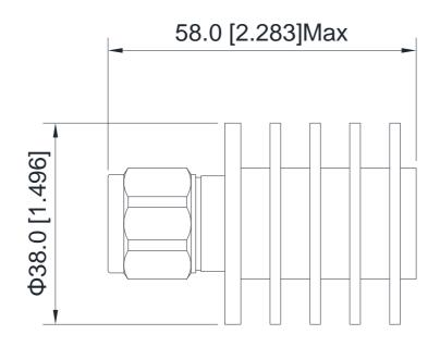
Unit: mm/ inch, General part tolerance is  $\pm 2\%$  unless otherwise stated.
