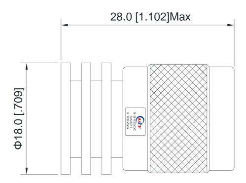
Unit: mm/ inch, General part tolerance is  $\pm 2\%$  unless otherwise stated.
