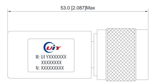
Unit: mm/ inch, General part tolerance is  $\pm 2\%$  unless otherwise stated.
