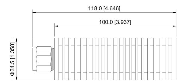
Unit: mm/ inch, General part tolerance is  $\pm 2\%$  unless otherwise stated.
