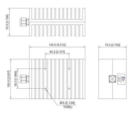
Unit: mm/ inch, General part tolerance is  $\pm 2\%$  unless otherwise stated.
