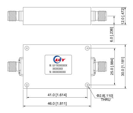
Unit: mm/ inch, General part tolerance is ±2% unless otherwise stated.
