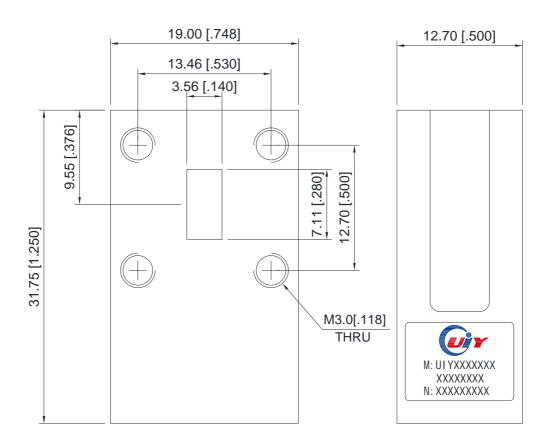
Unit: mm/ inch, General part tolerance is ±2% unless otherwise stated.
