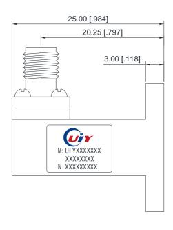
Unit: mm/ inch, General part tolerance is ±2% unless otherwise stated.
